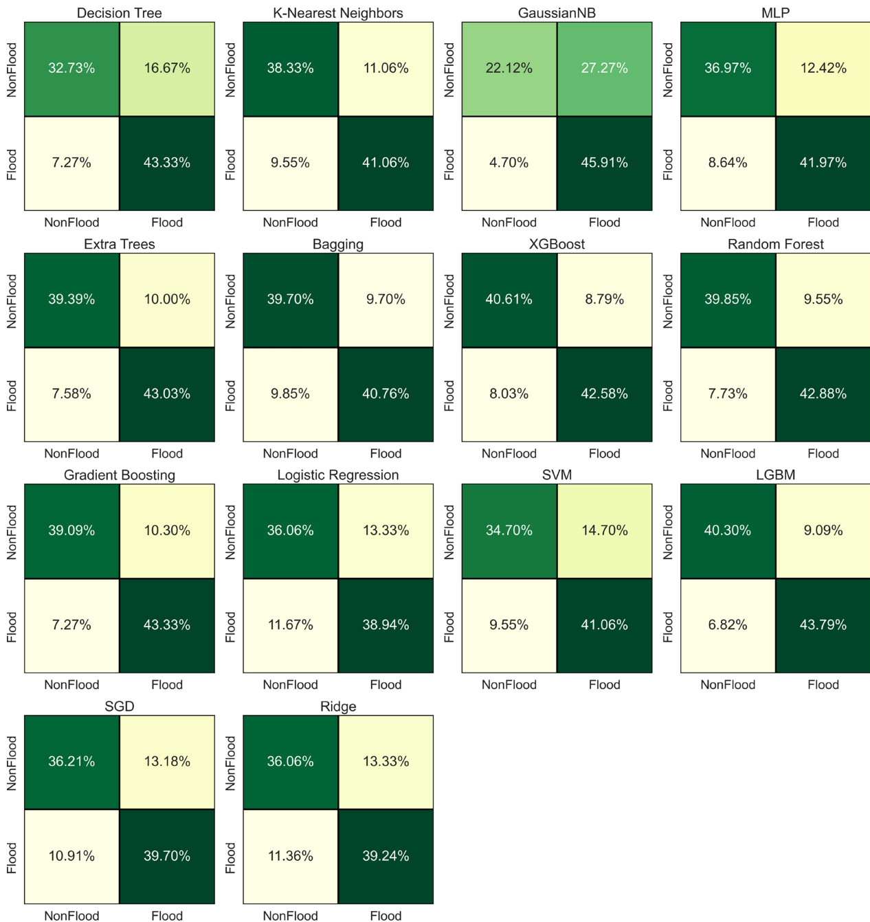
FIGURE 6 Confusion matrix for each ML model. In each confusion matrix, the left horizontal rows show the actual percentage of samples, whereas the bottom vertical columns show the predicted percentage of samples. The top left section in the matrix indicates the correct classified non-flood pixels and is called true negative (TN). The top right section shows the incorrect classified non-flood into flood class and is called false positive (FP). Similarly, the bottom left, and right sections show false negative (FN) and true positive (TP) values, respectively.
